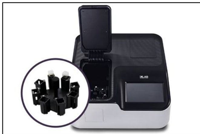
[Figure 1]. Alpha UV-Vis spectrophotometer - The Alpha is a double-beam UV-Vis spectrophotometer operating over a wavelength range of 190-1,100 nm, suitable for precise absorbance measurements and quantitative analysis. It is compatible with various cell-holder configurations, including a multi-cell holder, enabling sequential measurement of multiple samples, and in this study the absorbance of samples was measured at 765 nm for total polyphenol analysis according to ISO 14502-1.
