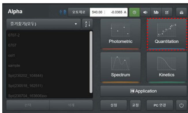
[Figure 2]. Main screen of the K LAB UV-Vis spectrophotometer - The instrument provides Photometric, Quantitation, Spectrum, and Kinetics modes, and in this study the [Quantitation] mode was used to perform total polyphenol analysis
