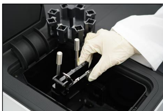
[Figure 3]. Tool-free cell-holder replacement mechanism of the Alpha UV-Vis Spectrophotometer - Ensures consistent mechanical referencing during holder removal and installation.
