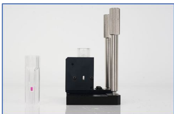
[Figure 2]. Micro Cuvette (BRAND GMBH, Cat. no: 759200) and POP's Microvolume Cell Holder. The POP is equipped with a standard 8-cell multi-cell holder but is also compatible with various accessories, including the Microvolume Cell Holder, allowing for flexible experimental configurations.
